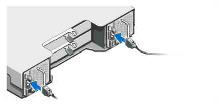
Figure 2. Connecting the Power Cable(s)
